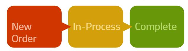
The Ship/FX Pack Station employs advanced HMI design technology to simplify operations. The entire interface is color-coded to guide and prompt users through the shipping process. At the start of each new transaction, fields are red to indicate their incomplete status. As users input data these fields turn gold. When all fields are green, labels may be printed to complete the shipping process.
